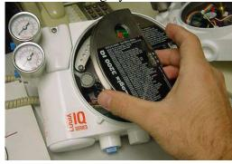
3. Attach wires from the Low Profile Position Sensor Module's terminal strip to the 3200IQ/MD terminal strip; 22 or 24 AWG wire is recommended. Be sure to run the wires through the threaded conduits and to connect terminal A to terminal A, B to B, and C to C.
